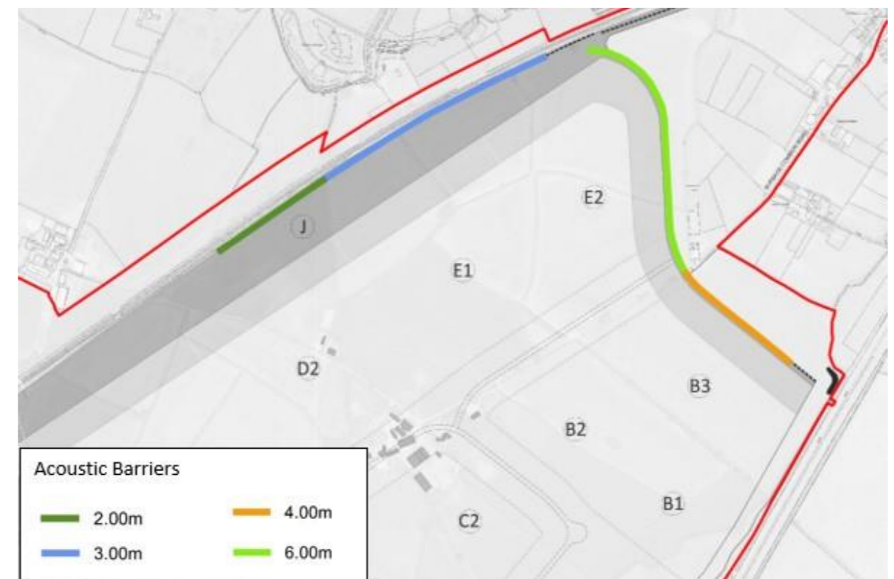
Fig. 63 Proposed Noise Barriers to north west of Railport and to the north east of head shunt (Document Reference 6.3.10.10)
